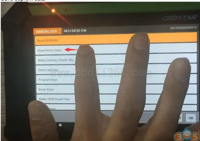
Read IMMO data Switch ignition on Reading data Immo indicator will flash during this procedure
