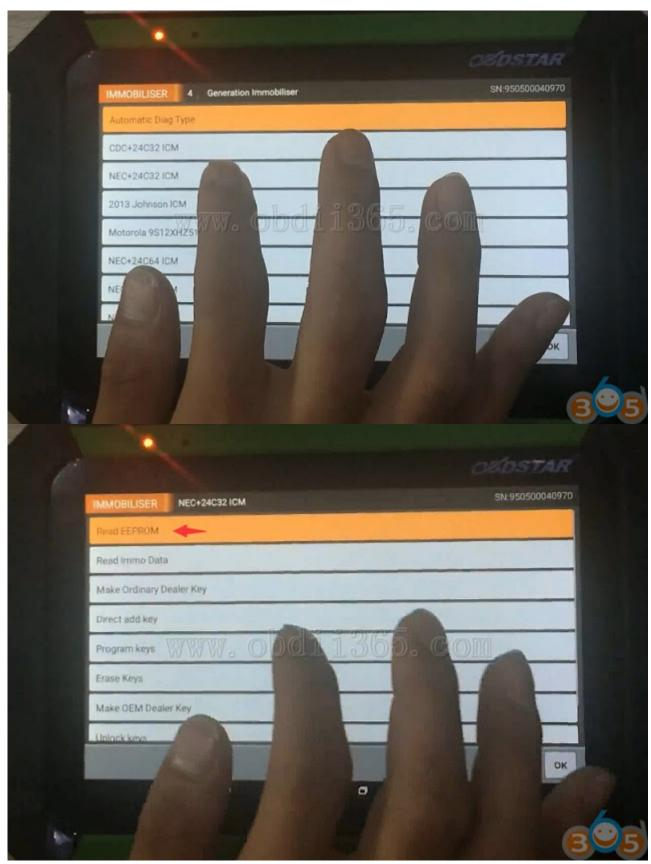
Read EEPROM data Turn ignition to ON position Reading data Immo indicator will flash during this procedure
